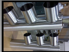
Clean Tube Welds
